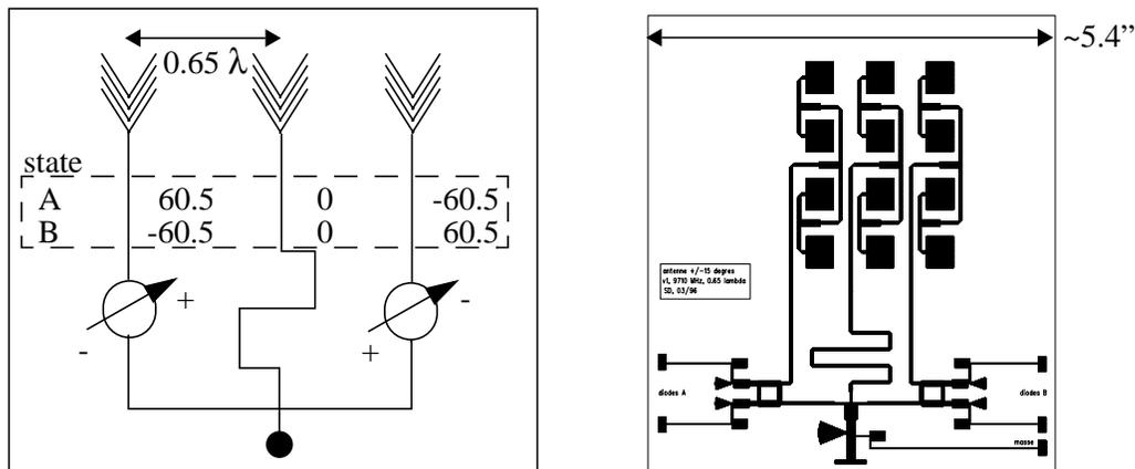
Figure 1. Schematic of the phased array antenna and final layout representation.
