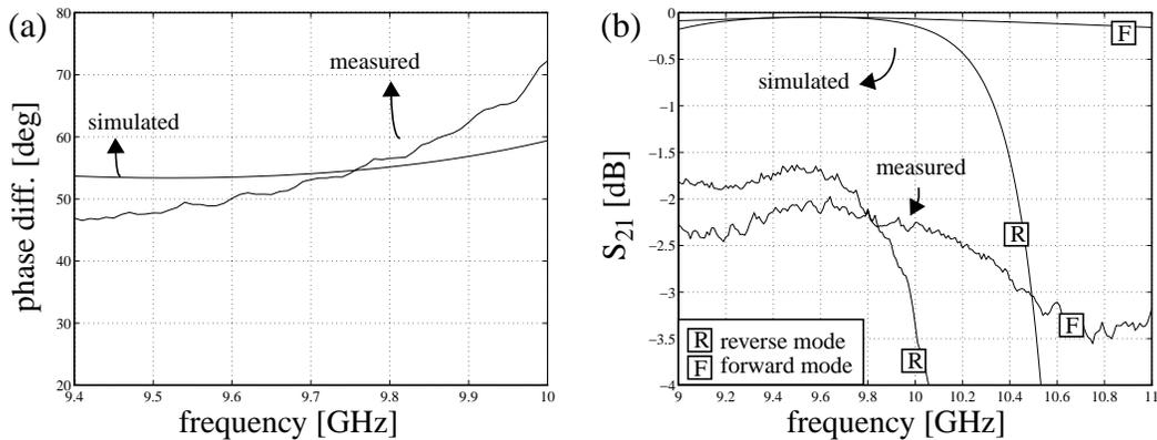
Figure 6. Loaded line phase shifter: (a) simulation and measurement of phase difference between states; (b)  $S_{21}$  simulation and measurement in both states.
