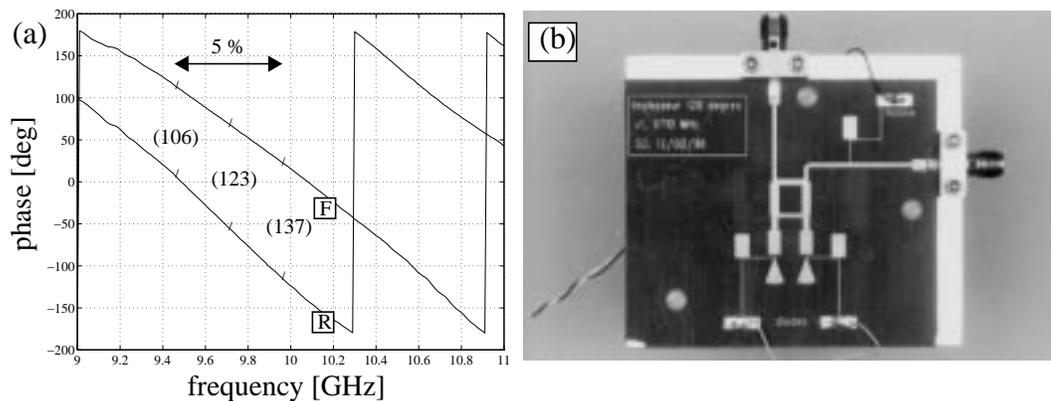
Figure 5. Reflection phase shifter: (a) phase as a function of frequency for both states; (b) photograph of the phase shifter.
