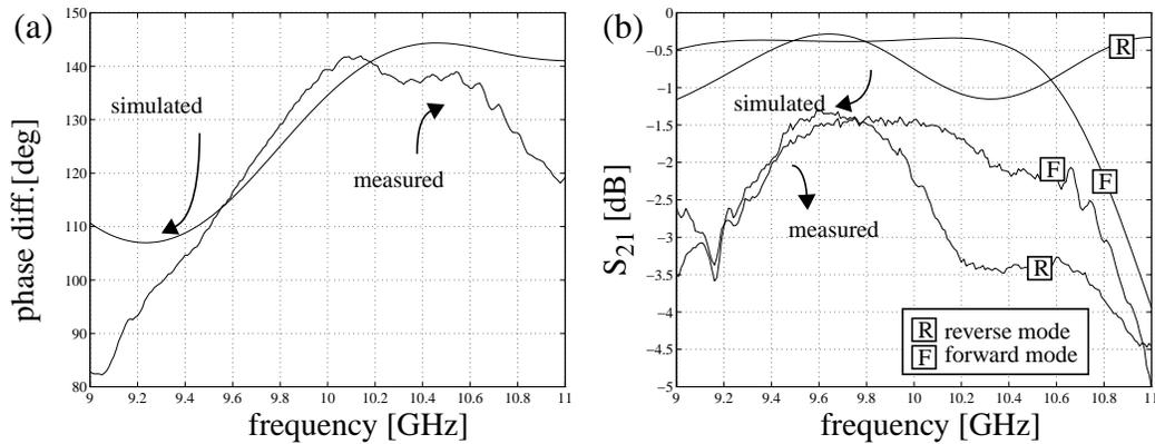
Figure 4. Phase shifter performances: (a) simulation and measurement of phase difference between states; (b)  $S_{21}$  simulation and measurement in both states.
