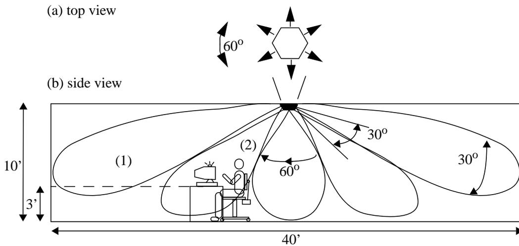
Figure 2. Antenna topology in a typical room
