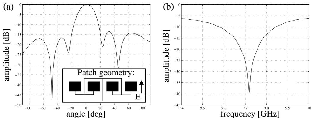
Figure 3. A 4 by 1 antenna measurements: (a) radiation pattern in the H plane; (b) reflexion coefficient.
