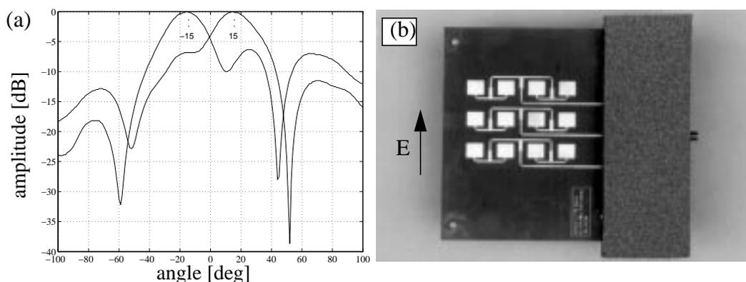
Figure 8. (a) Measured radiation pattern in the E plane for both states; (b) photograph of the measured antenna.
