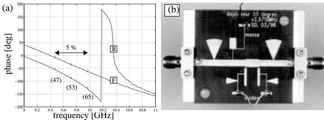
Figure 7. Loaded line phase shifter: (a) phase as a function of frequency for both states; (b) photograph of the phase shifter.
