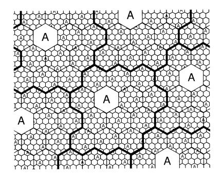
**Fig. 1**: A typical frequency double reuse system. The large "A" show the macrocells where the frequency A is used. The small "A" show the microcells where the frequency A is reused with low power for the indoor cellular system.
